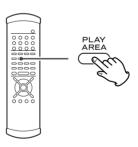
When playback is stopped, use the PLAY AREA button to select the playback area. Some DVD audio discs have DVD video areas which can be accessed through this function. Additionally, SACD discs may contain two or more separate audio areas, selectable in this way.
